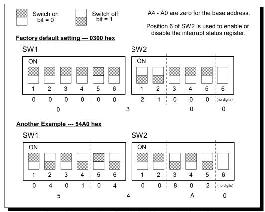
Figure 5 --- Serial Port base I/O address selection switches
